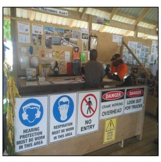
Figure 21: Display of Process Plant Hazards and Site Specific PPE
