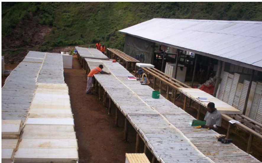
Figure 2: Core logging at Yandera project camp
