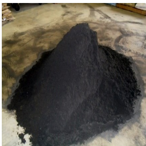
Zircon concentrate at a grade of 66.2% ZrO 2
