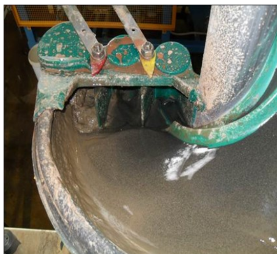
Bulk sample heavy mineral on spiral separator magnet
