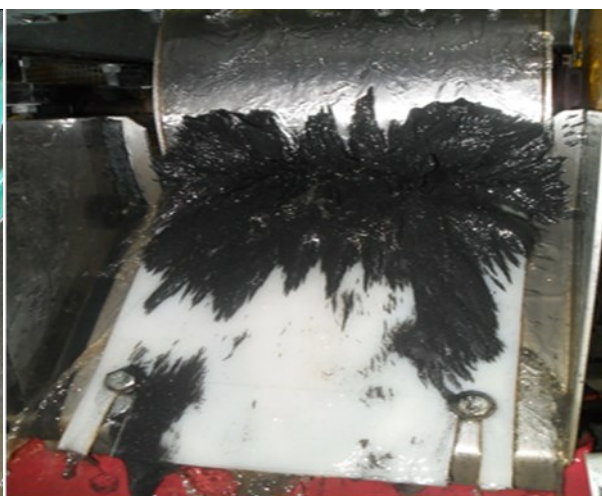
Extracting magnetite from heavy mineral using drum
