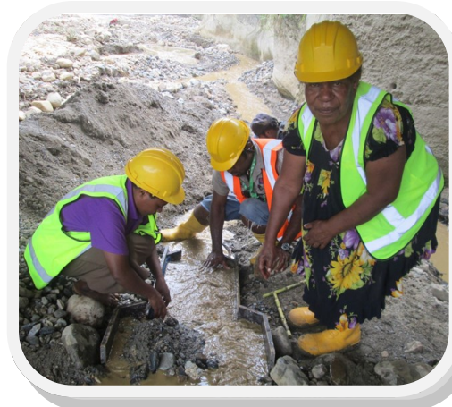
Level 1 participants learn the basics of sluicing using a simple sluice box in Level 1 practical training.
